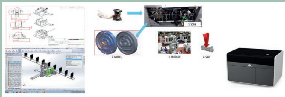
Figure 10.11: Capturing parts shapes from CAD systems or physical scanning, then outputting a replacement part on a local 3D printer
